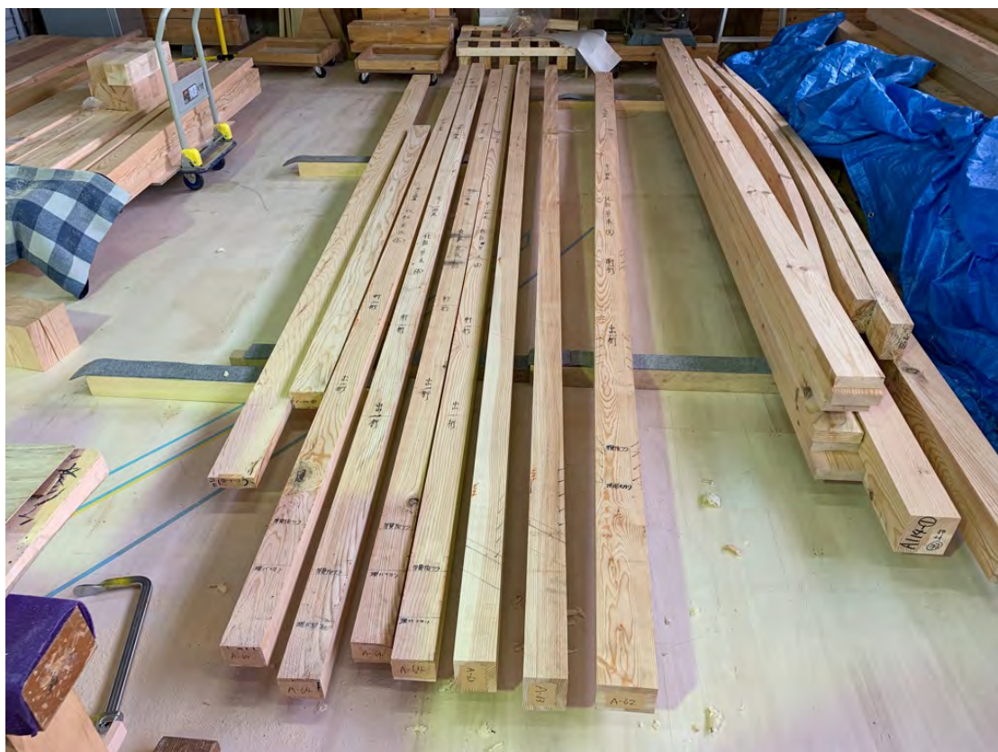
The timbers that started marking and processing. 【upper photo: timbers for roof truss, lower photo: timbers for rafter】
