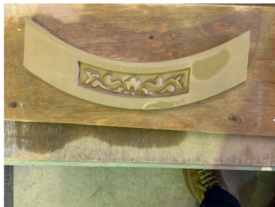
Checking the design of gatou (the tip of the eaves-end tile) and making corrections.
