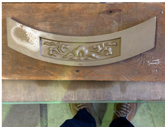
Checking the design of gatou (the tip of the eaves-end tile) and making corrections.
