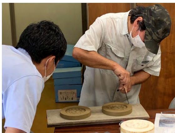
Checking the design of gatou (the tip of the eaves-end tile) and making corrections.
