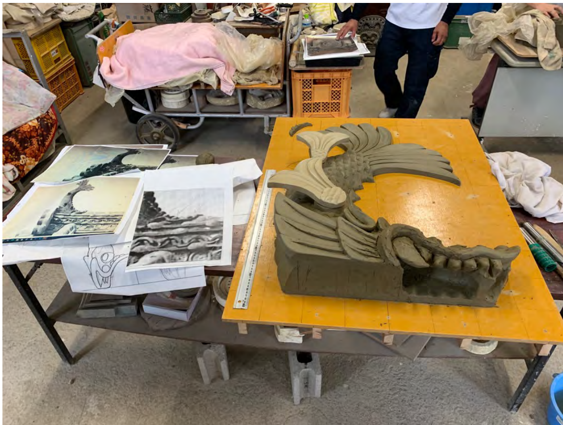
The clay mold to confirm the design of shachigawara restored from the old photographs.
