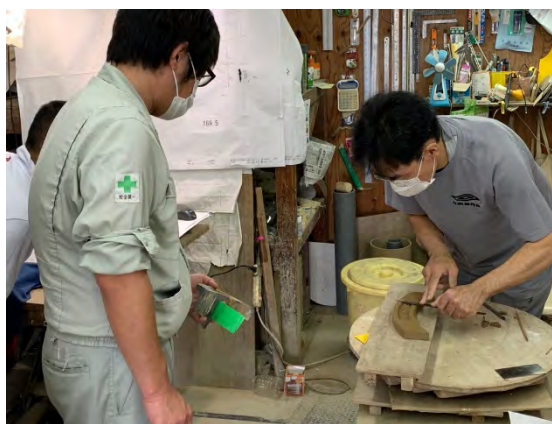
Checking the design of gatou (the tip of the eaves-end tile) and making corrections.
