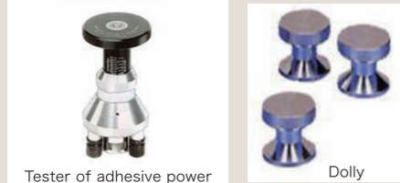
Epoxy adhesive is used to bond the paint film surface, and the adhesive force of the paint film is measured with an adhesion tester.
