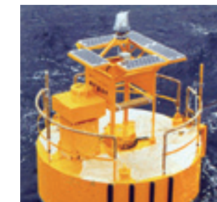
Ocean ranch using an acoustic feeding system
