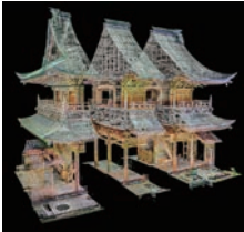
Point cloud data of Sanmon gate (both exterior and interior displayed simultaneously) Eihei-ji and Shimizu Corporation joint inspection Survey collaboration T&I 3D
