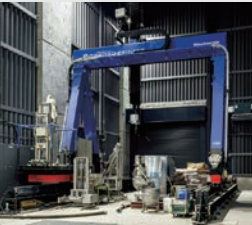
Largest construction 3D printer in Japan
