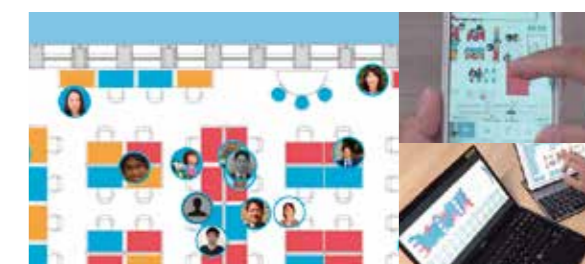
Positioning data system: A PC or smartphone can be used to confirm the locations of individuals on a diagram of the floor layout in real time, both from within and outside of the company
