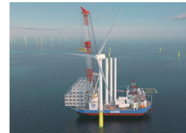
Image of Self-Propelled SEP vessel to be constructed (attaching blades)
