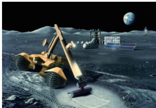
Conceptual drawing of heavy robotic equipment excavating the lunar surface by remote control
