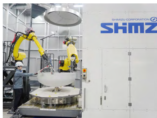
Manufacturing a large tank with a diameter of 1.5 meters using a metal 3D additive manufacturing system
