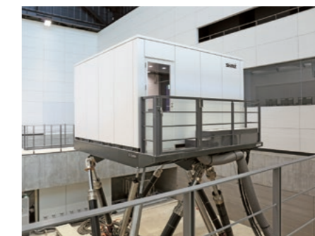
The "E-Spider" large-stroke shaking table fitted with a cabin
