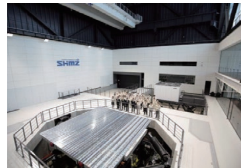
The "E-Beetle" large-scale shaking table
