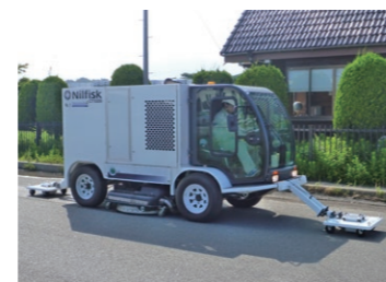
A pressure-hose truck equipped with the high-efficiency decontamination system *1
