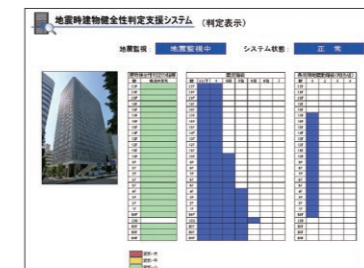
Example of a seismic monitoring system screen
